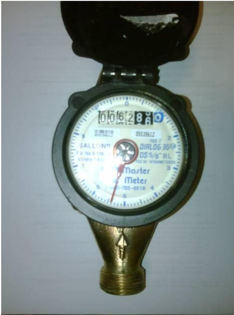
For example, the meter reading on the picture above is **62,865** gallons.
